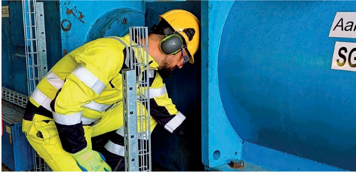
Bram Vervisch of Orbits while measuring strike-throughs due to bearing currents. (©Orbits)
